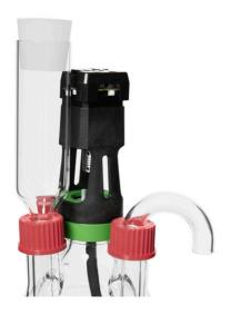
BRS III is a laboratory-scale instrument designed to replicate continuously fed anaerobic fermentation processes with full automation, user-friendly operation, and reliable performance. Featuring nine parallel channels, it allows simultaneous testing of multiple process conditions, making it a powerful tool for optimising biogas production.
